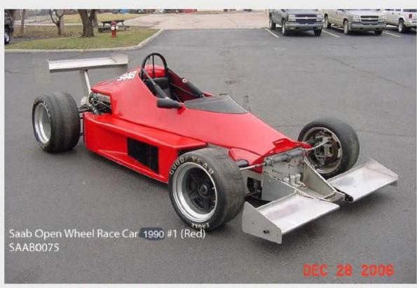
Since all the cars used Saab engines reliability was more important than high performance. The engines were basically stock 1985 cc 16-valve twincam turbo engines with an output of 225 hp. They differed from street versions in that the boost is increased, emission control systems are removed, fuel-injection settings revised and a racing exhaust fitted, together with dry-sump lubrication. By 1991 the marketing strategy at Saab changed and Saab US did little more than provide the engines.
